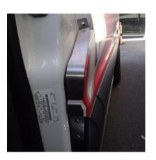
8. Now that Door Guard is in position and clears gas door and driver's door you can add third screw at top of Door Guard. Check for clearance again.
