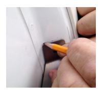
4. Using a pencil draw a line at the top of the Door Guard on the Transit body so when you remove the backing of the double sided tape you will know where to place it.
