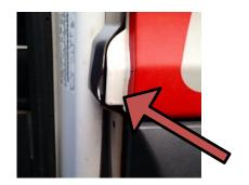
1. Place Door Guard so it lines up with lip of gas door and up against the plasitic trim where the bottom two holes are in the Door Gaurd.
