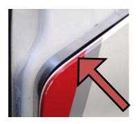
6. Check again for clearance with the gas door and the Door Guard you can bend and move the Door Guard a small amount if you need to adjust for clearance or remove one end of the double sided tape to reposition.
