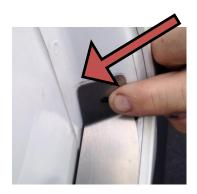
3. Postion top of Door Gaurd with finger in corner of body and open and close gas door to make sure door clears gas door guard. You want to postion it as close as possiable to gas door, but NOT TOUCHING.
