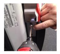
2.Using a screw gun or similar device to install the two lower screws.
