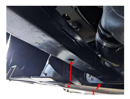
**4.** Next, continue following the frame rail back until you reach the cross-member. For this 3<sup>rd</sup> mounting hole you will need to remove the inner of the two M8 bolts on both frame rails.
