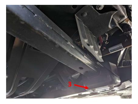
**5.** Using the supplied M8-1.25x30 bolts and machined aluminum washers, replace the factory bolts and install the skid plate starting with the 3<sup>rd</sup> mounting location. Tighten the bolts to 24Nm.
