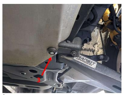
**6.** Now install the M8-1.25x100 bolts and machined aluminum washers through the skid plate and frame rails at the 1<sup>st</sup> and 2<sup>nd</sup> mounting locations. Then install the supplied M8 nuts and flat washers on the top section of the frame rails. Tighten the bolts to 24Nm.
