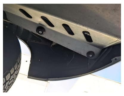
**7.** Finally. Torque down the M8 button head bolts joining the two halves of the skid plate together to 24Nm.
