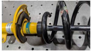
6. Install the provided spring spacer in the following position. Once re-assembled the strut should look like the picture on the right.
