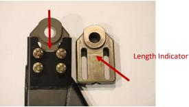
11. After installation of the kit, the toe and camber **MUST** be adjusted. DO NOT DRIVE WITHOUT TOE ADJUST!
