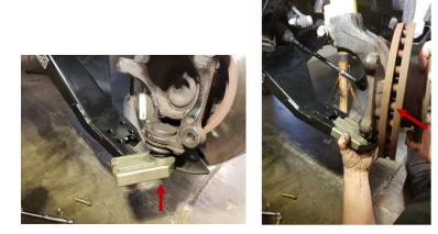
8. Once the adjuster block is fully inserted Slide the four #3 bolts and #1 washers in from the top of the control arm and through the adjuster block. Attach the four #2 washers and #4 nuts from the bottom of the control arm.
