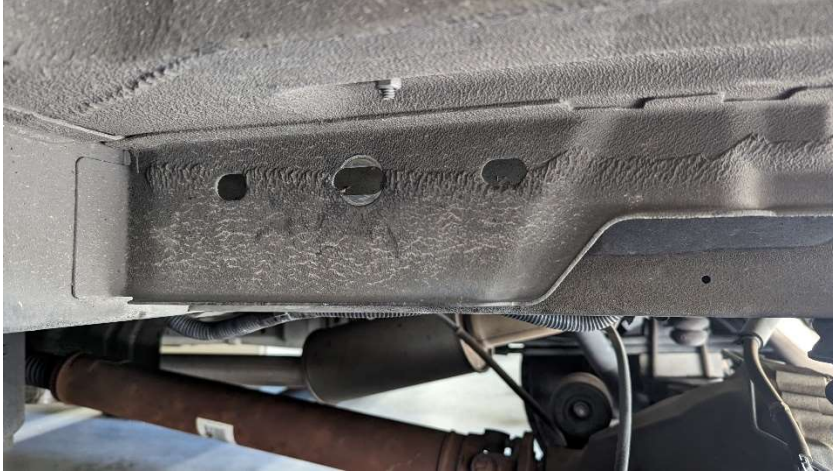
Before installing reinforcement plate
